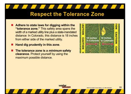
Respecting the tolerance zone protects buried utility lines from damage and also protects you from injury.
