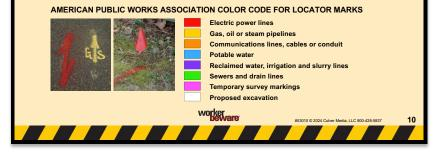
After you contact 811, the underground utility locator service will arrange for each member utility to send someone out to your dig site to mark the underground lines.
